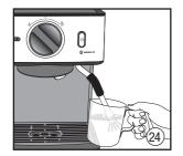
Angle jug to rest steam wand on spout and place nozzle just below surface of the milk.
